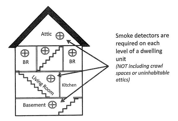
Smoke Detectors may be placed on walls, but must be higher than any opening into the room (e.g. doors, windows) and are placed between 4" and 12" from the ceiling.
